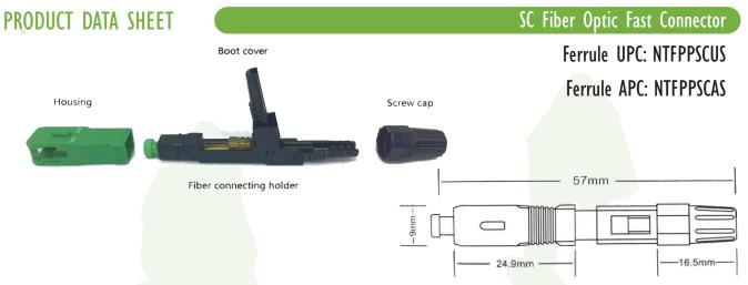
Optical fast connector takes use of the latest generation of Rapid Ready-Terminal technology. After terminating, both the optical and mechanical performances reach the standard for patchcord and meet the demand for making patchcord on site by mechanical splicing.
