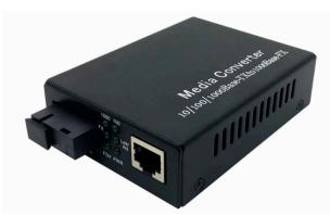
Easy to set-up and install, this compact, value-conscious fast Ethernet media converter features auto-switching MDI and MDI-X support on the RJ45 UTP connections as well as manual controls for UTP mode, speed, full and half duplex.
