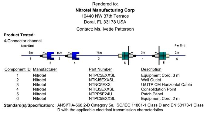
Product(s) Literature May Include: ETL Verified 4-Connector Channel to ANSI/TIA-568.2-D Category 5e, ISO/IEC 11801-1 Class D and EN 50173-1 Class D, along with channel illustration, and parts numbers.
