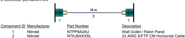
Standard(s)/Specification: ANSI/TIA-568.2-D Category 6A with the applicable electrical transmission characteristics
